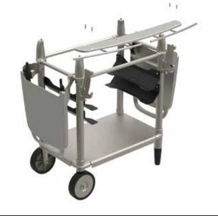
**STEP 2.** Affix BELLY BAR WIRE to BELLY BAR SHELF using 5mm hex wrench (8X: 5mm X 18 mm long stainless steel countersunk machine screws)
