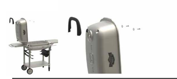
**STEP 2.** Open the UPPER CAPSULE into the open position and affix the handle using a no. 3 Phillips head screwdriver and supplied screws and lock washers as shown. Securely tighten screws.
