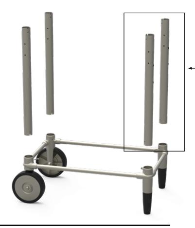
**STEP 3.** Place four VERTICAL TUBES into the corner lugs of LOWER CART TUBE ASSEMBLY. See Diagram for proper orientation.
