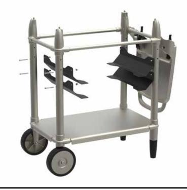
**STEP 8.** Affix SPEED RACKS to vertical bars on stand using 5mm hex wrench (8X: 5 mm X 45 mm long stainless steel machine screw, 8X: Stainless Steel Cap nuts)
