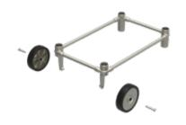
**STEP 1.** Affix wheels to LOWER CART TUBE ASSEMBLY using two axle screws and 5mm hex wrench. Ensure axle screws are tight.
