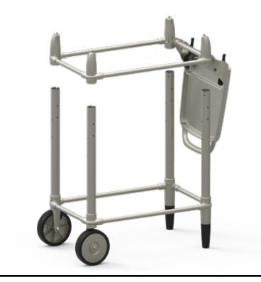
**STEP 5.** Place UPPER CART TUBE ASSEMBLY on top of the four VERTICAL TUBES as shown. The SHELF should be oriented on the side opposite the wheels.
