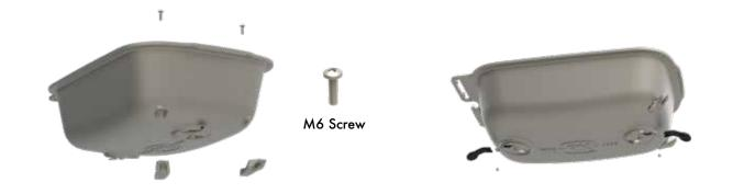
**STEP 1a.** Attach SHELF LOCKS to LOWER CAPSULE oriented as shown using provided M6 screws and lock washers. NOTE: If provided in box, apply optional thread lock material to threads prior to fastening. Otherwise, disregard. **STEP 1b.** Attach VENT HANDLES to LOWER RADIAL VENTS using provided M6 screws. Handles are identical, so work interchangeably with VENTS.
