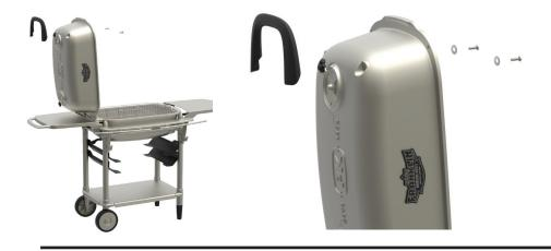
**STEP 2.** Open the UPPER CAPSULE into the open position and affix the handle using a Phillips head screwdriver and supplied screws and lock washers (hadrware bag E) as shown. Securely tighten screws.
