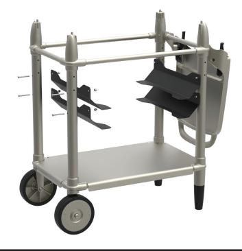
**STEP 8.** Affix SPEED RACKS to vertical bars on stand using 5mm hex wrench (8) 5 mm X 45 mm long stainless steel machine screw, (8) Stainless Steel Cap nuts (hardware bag F).
