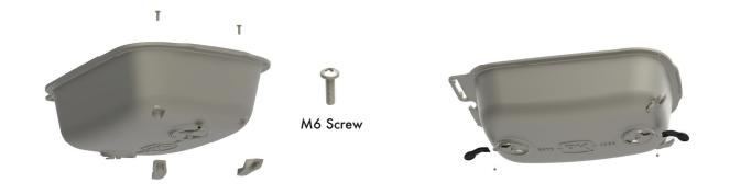
**STEP 1a.** Attach SHELF LOCKS to LOWER CAPSULE oriented as shown using provided M6 screws and lock washers (hardware bag C).
