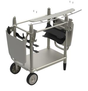
**STEP 2.** Affix BELLY BAR WIRE to BELLY BAR SHELF using 5mm hex wrench (8) 5mm X 18 mm long stainless steel countersunk machine screws (hardware bag I).
