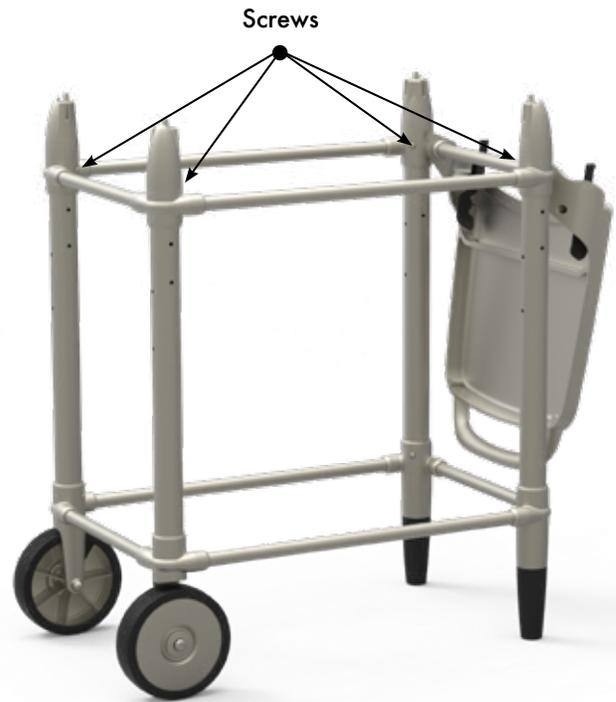
**STEP 6.** Affix VERTICAL TUBES to UPPER CART TUBE ASSEMBLY using provided hex screws and 4mm hex wrench. **Do not fully tighten hex screws at this step.**
