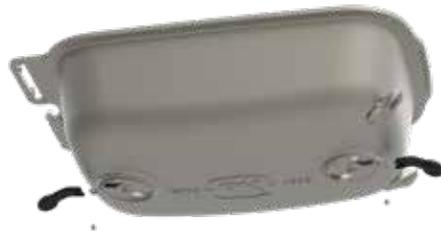
**STEP 1a.** Attach SHELF LOCKS to LOWER CAPSULE oriented as shown using provided M6 screws and lock washers. NOTE: If provided in box, apply optional thread lock material to threads prior to fastening. Otherwise, disregard.
