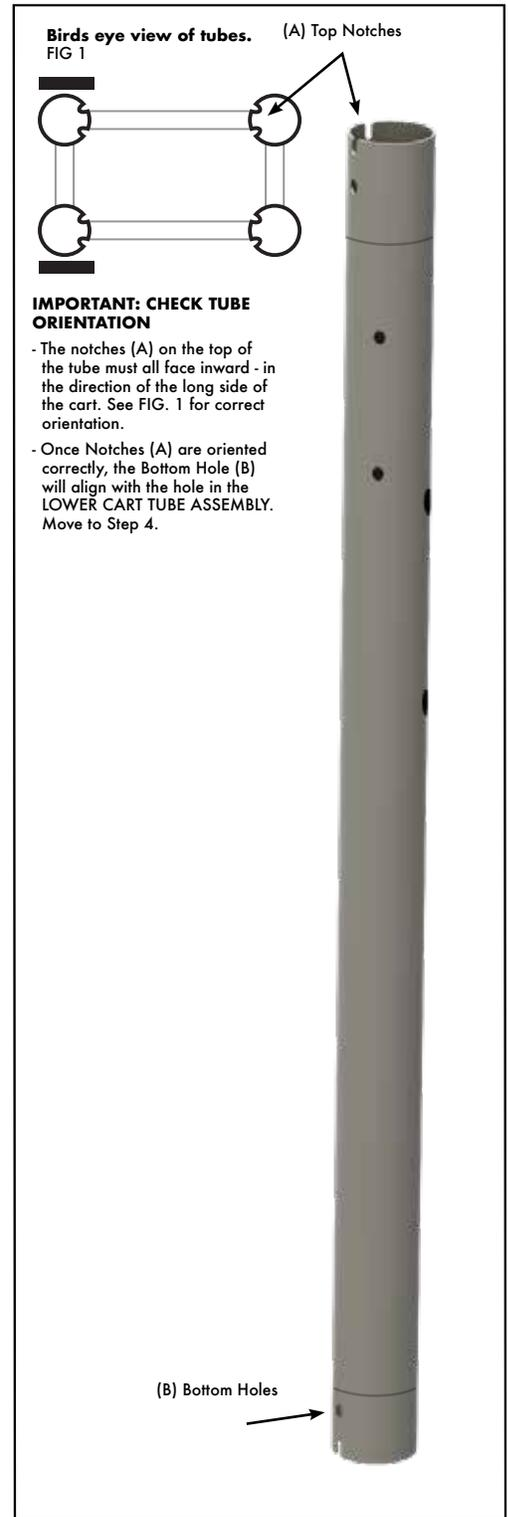
**STEP 3.** Place four VERTICAL TUBES into the corner lugs of LOWER CART TUBE ASSEMBLY. See Diagram for proper orientation.
