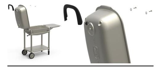
**STEP 2.** Open the UPPER CAPSULE into the open position and affix the handle using a Phillips head screwdriver and supplied screws and lock washers (hadrware bag E) as shown. Securely tighten screws.
