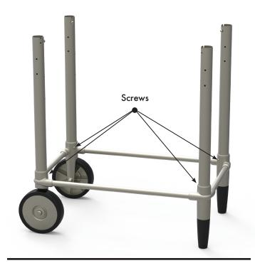
**STEP 4.** Affix VERTICAL TUBES to LOWER CART TUBE ASSEMBLY using provided hex screws (hardware bag B) and 4mm hex wrench. Do not fully tighten.
