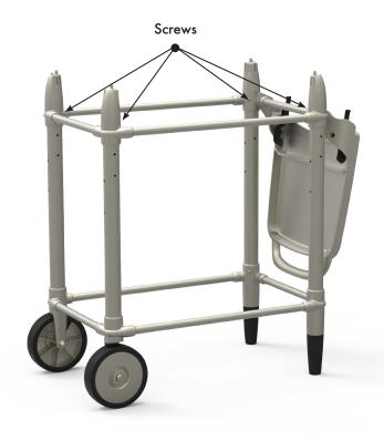
**STEP 5.** Place UPPER CART TUBE ASSEMBLY on top of the four VERTICAL TUBES as shown. The SHELF should be oriented on the side opposite the wheels.
